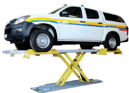
Standard lifting by wheel lifting supports
