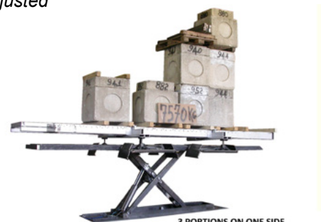
LOAD TEST ON RUBBER BLOCKS AND + 50% OVERLOAD EN 1493 EUROPEAN STANDARD 3 PORTIONS ON ONE SIDE 1 PORTION ON THE OPPOSITE SIDE
