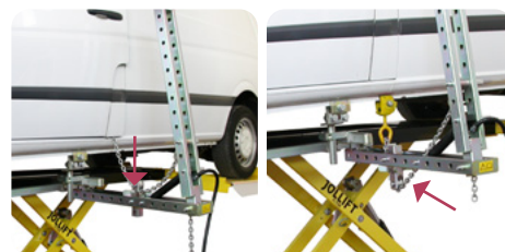
3. Telescopic chain deviation roller with pivot (1 pc)
