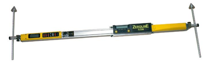
Zeroline – length, width, diagonal and height are measured digitally with a numerical accuracy. Zeroline can work with any inclination – by pressing the calibration button you create the zero reference plane even if the car is not in a horizontal position Suitable for measuring body / front end assembly / wheel alignment etc.
